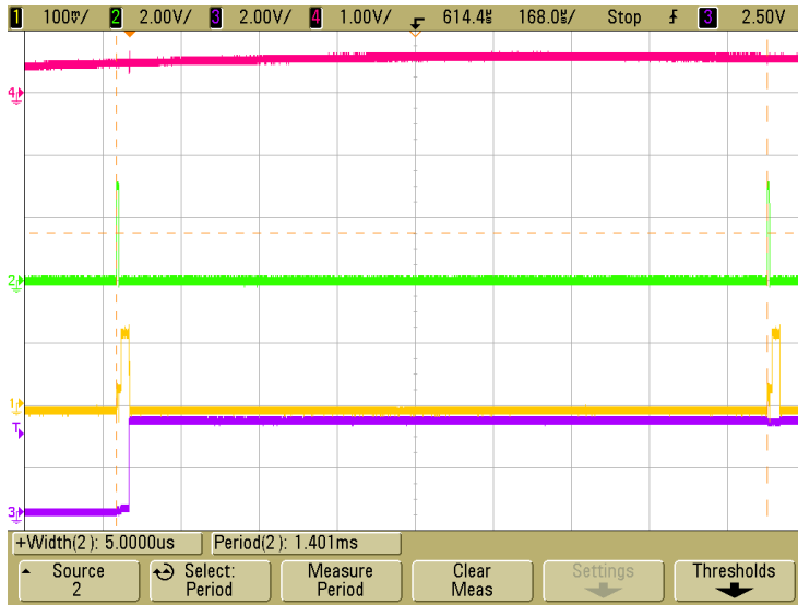
Figure 11 - Slower Sampling Mode – measured TE1 and TE2
